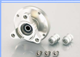
FRONT HUB for 173 mm pitch wheel WITHOUT OFFSET (SILVER) 500-1083220 (BLACK) 500-1083230 ※ WAVE DISC ROTOR is NOT useable.
